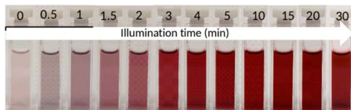
Figure 1. Reduction of gold through UV illumination of an hybrid imogolite dispersion.
